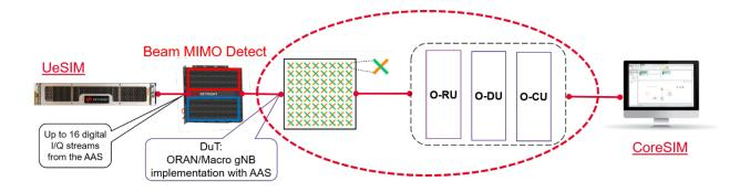
Up to 64 separate bidirectional radio ports operating in FR1 up to 5GHz TDD bands can be used with different MU-MIMO configurations.
