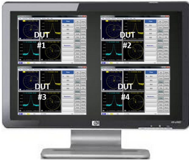
Figure 5. Multiple instances of the M937XA software are launched with each instance behaving as an independent instrument to be used simultaneously.
