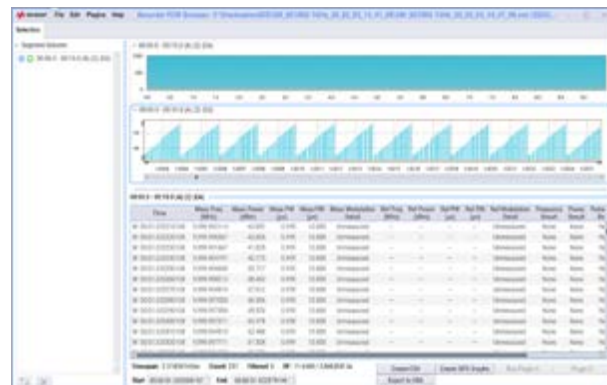
Figure 9. PDW browser containing a histogram of all pulses, a short power pulse, and a table of easily filterable pulse attributes
