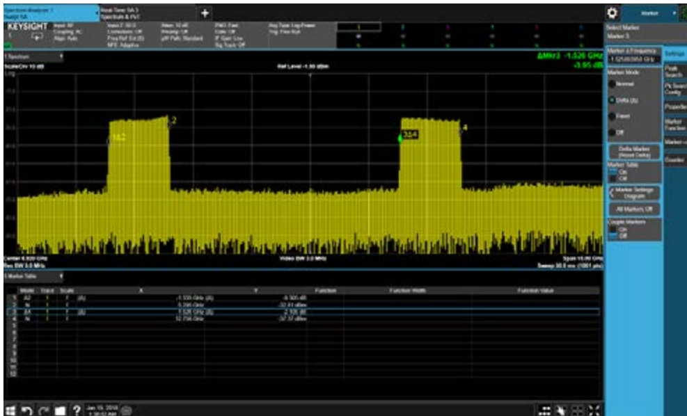
Figure 4. Two 1.5 GHz wide LFM chirped emitters 7 GHz apart from one UXG source UXG source
